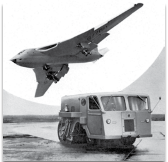
Runway sweeper which had a capability of moving at 12mph to effectively clear debris and surface water. The swooping aircraft is a Victor bomber that was introduced in 1958 and retired in 1993. Ironically given the subject matter, the Victor was modified as an in-flight refuelling aircraft.
