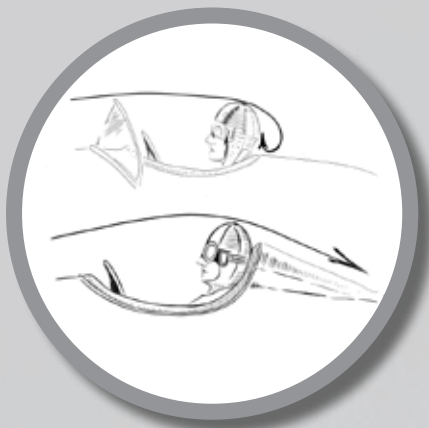
How airflow and drag are affected by cockpit design (credit: Scott Cullen)
